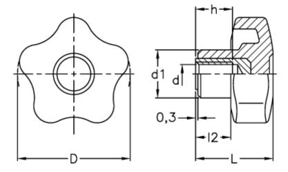
$$\begin{array}{ll} D & = 25 \\ d1 & = 13 \\ d \ 6H = M5 \\ h & = 10 \\ L & = 19 \\ l2 & = 8 \end{array}$$
